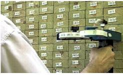
The TIMBER TAGGER is easily mounted on a light wire pneumatic staple gun. It is designed and engineered to apply millions and millions of Timber Tagger Tags. When the staple gun needs cleaning or repair, the TIMBER TAGGER can easily be detached and mounted to another in seconds with only one screw.
