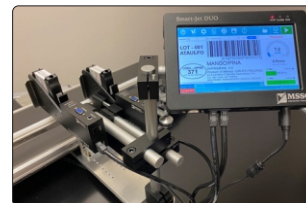
Connect up to 2 printheads at one time
